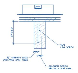
Figure 3. Typical Anchor with Lag Screw Attachment.
