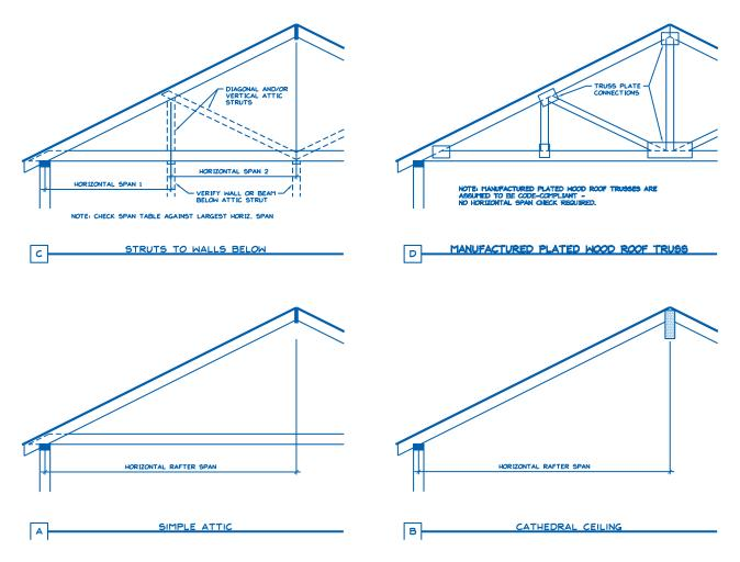
Figure 4. Definition of Rafter Horizontal Span.
