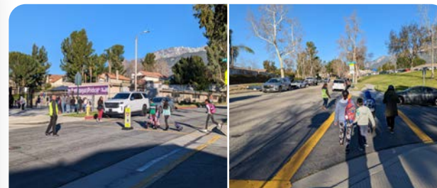
Curb extensions can shorten the crossing distance for students and visitors of Caryn Elementary School and an RRFB can enhance awareness of pedestrians within the crosswalk
