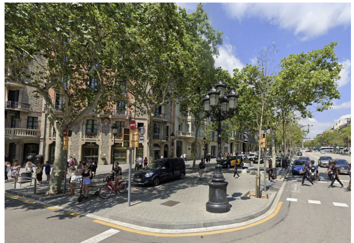
Frontage lane with raised crosswalk slows traffic, especially at intersections
