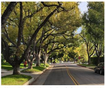
Wide, continuous planting strip allows for frequently spaced large trees with large canopies, providing lots of shade.
