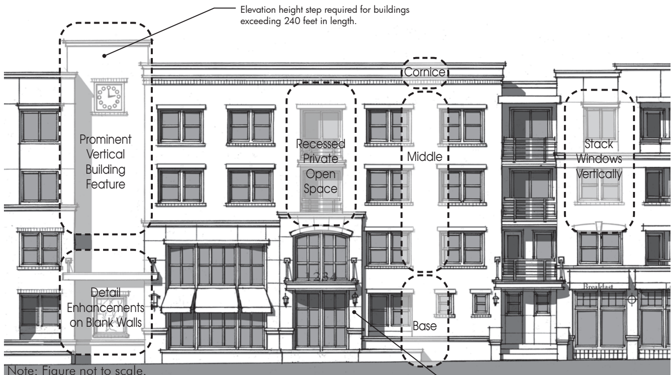
Figure 9.45: Massing and Articulation Diagram
