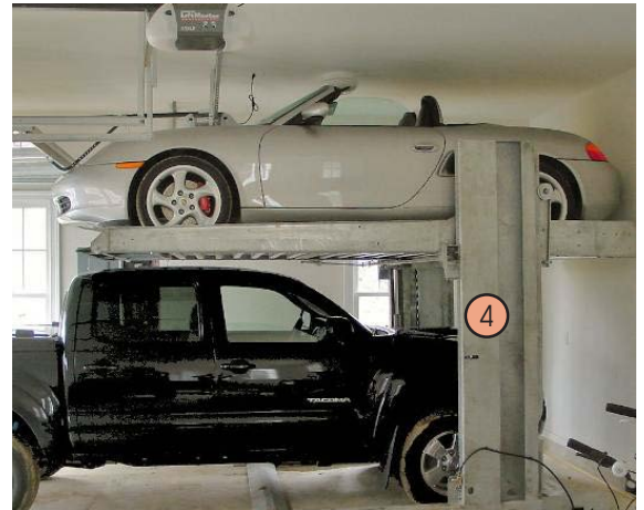
Car lift example, can be used in private garage or shared parking structures
