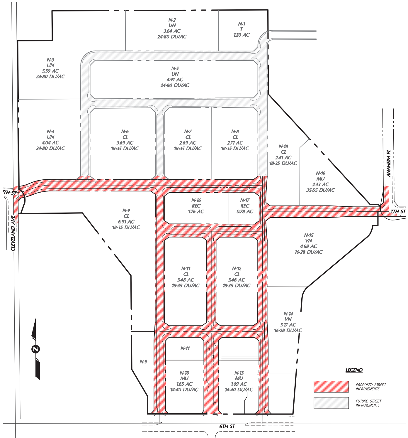
Figure A-22: Conceptual Phase 2 Street Improvement Facilities Plan
